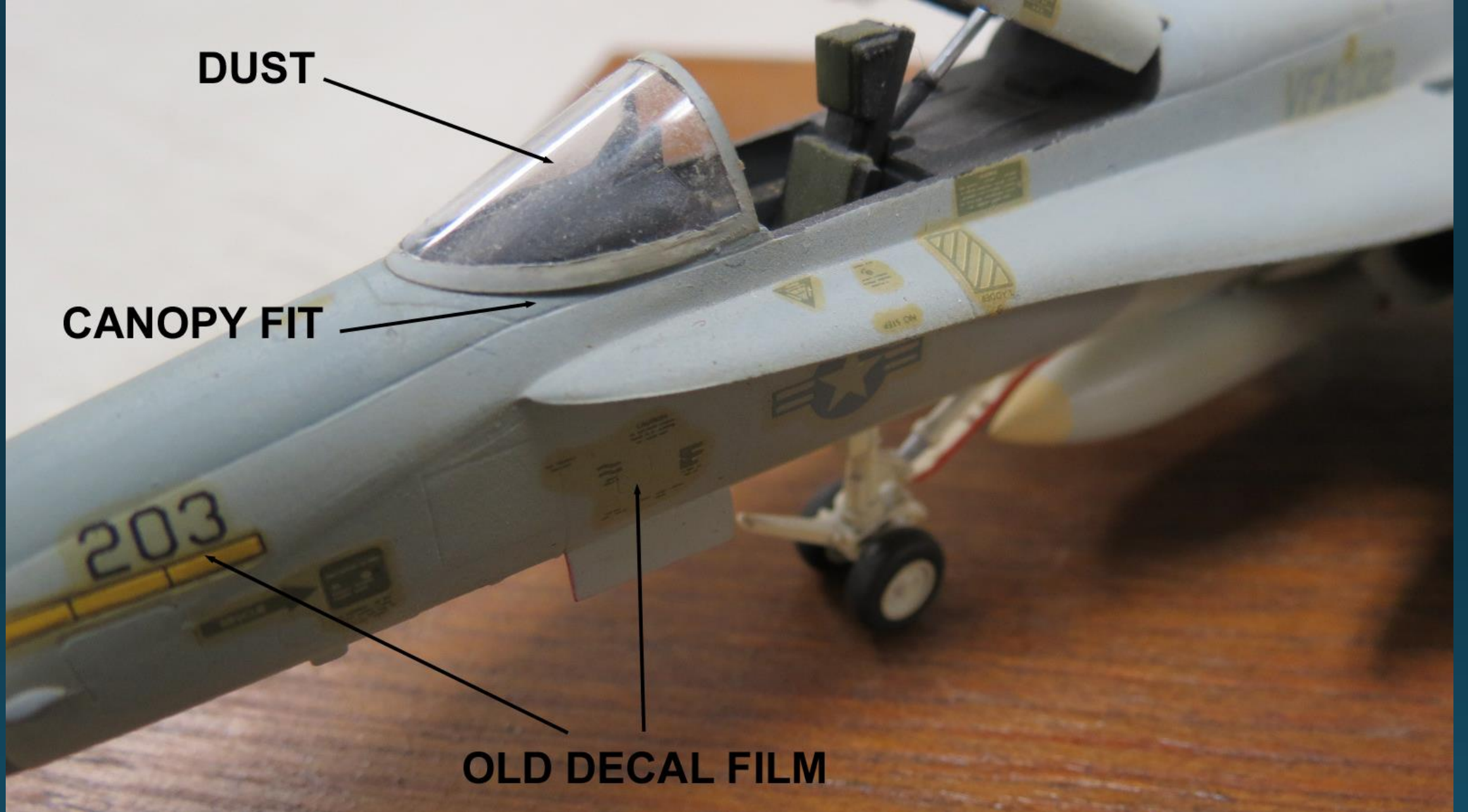
We can see yellowed decal film, poor canopy fit, and a dirty canopy.
